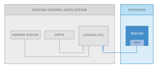
The connection of BioCon to your existing control system works via a standardized OPC interface to the central PLC.
