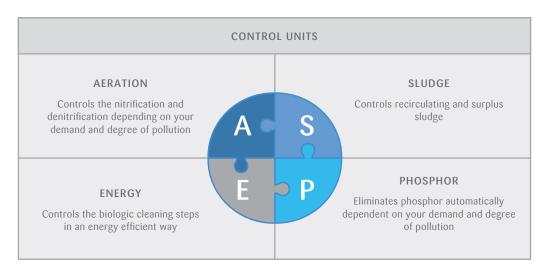
All BioCon components can be chosen separetly as required. The components interlink and BioCon combines them into a holistic controls strategy.
